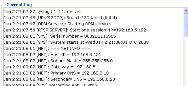
This column displays the system's log in chronological order. The system log is stored in the Network Camera's buffer area and will be overwritten when reaching a certain amount.
