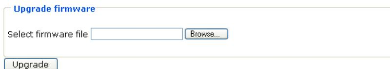
This feature allows you to upgrade the firmware on your Network Camera. It takes about five minutes to complete the process. Do not power down the Network Camera during the upgrade. The upgrade is successful as you see “Reboot system now!! This connection will close”.
